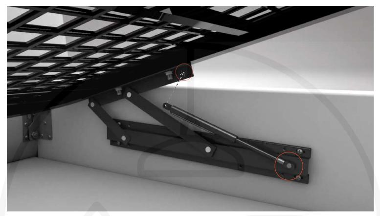
Attach the remaining piston to the hinge using the M8x15mm bolts in the locations shown above.
