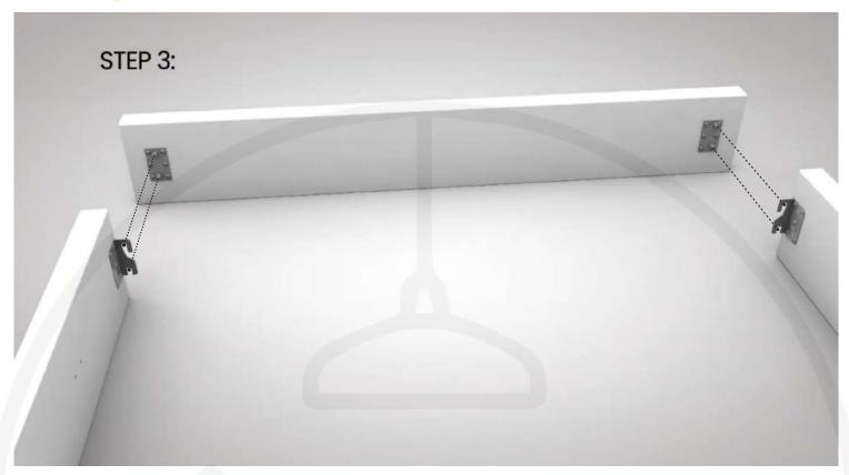
Attach the footboard to the siderails using the pre-fitted hook fixings, then tighten the nuts.
