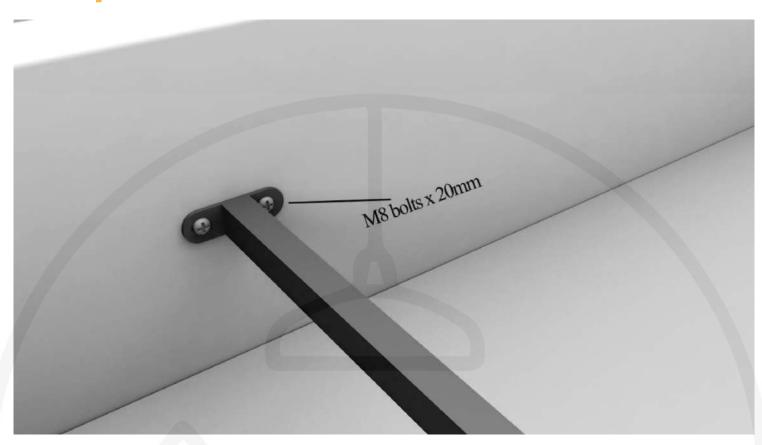
Secure the support bar using two M8x20mm bolts. Repeat this step on the other side of the bed.
