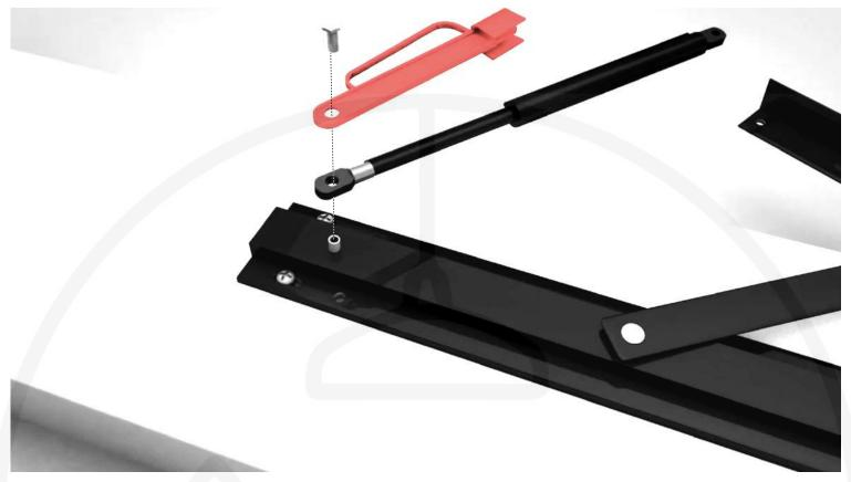
Use an M8x25mm long bolt to secure the components in the order shown above.
